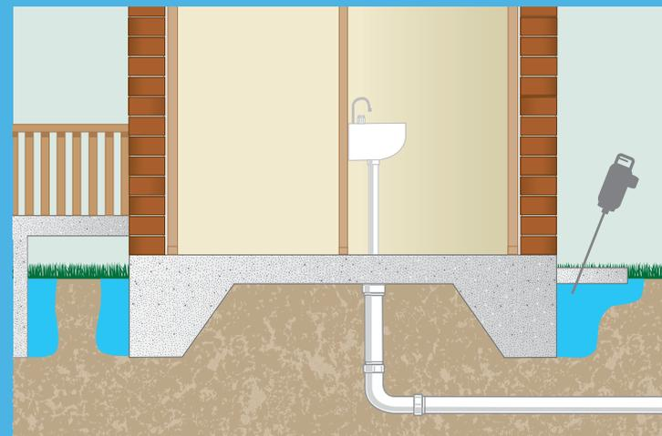
*Illustration 2: Shows the application of ALTRISSET to the soil around the exterior foundation.*
